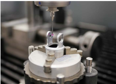
CMM inspection of finished part programmed in ESPRIT
