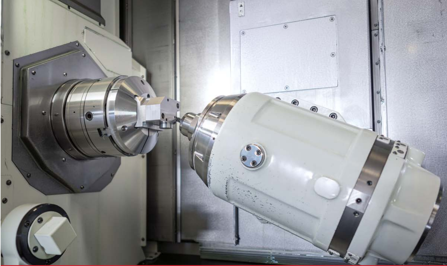
Machining a pavement marker on a MAZAK Integrex i200s 7-axis multi-tasking machine.
